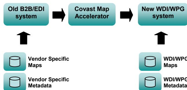
The Covast Map Accelerator creates WebSphere Data Interchange (WDI) or WebSphere Partner Gateway (WPG) document definition and map import files directly. The generated files can be imported into WebSphere using the WDI/DIS Client.
